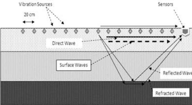
Fig 1: General Arrangement of field data Collection
