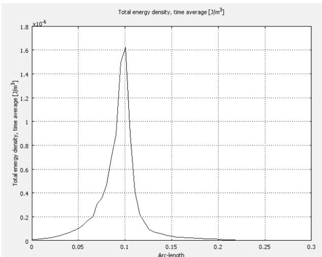
**Fig. 5** Energy density/arc length (835 MHz)
