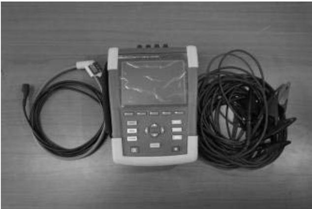
Fig.2. Flukemeter for Power quality indices measurement
