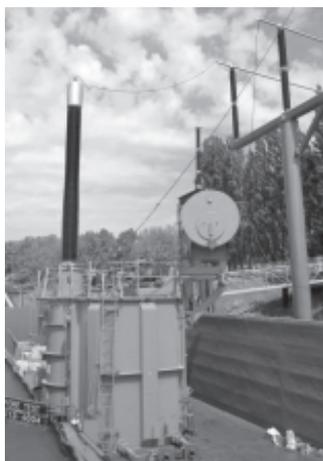
Fig. 6: Short-circuit test of a 800 kV class transformer
