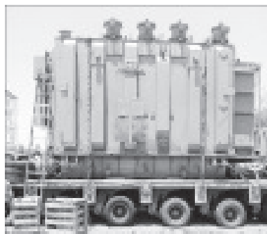
Fig.1: Transformer loaded on multi wheeled low bed Tractor Trolley
