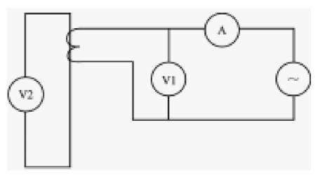
Figure 6 – Alternative connection for Ct ratio test
