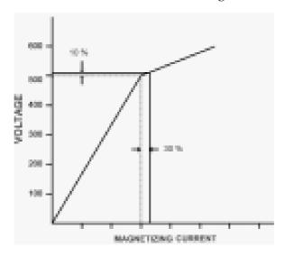
Figure 4 - Typical magnetization curve of current transformer
