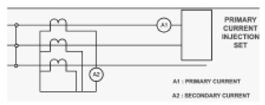
Figure 5 - Connection scheme for ratio test of current transformer
