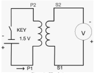
Figure 1 : CT polarity test setup
