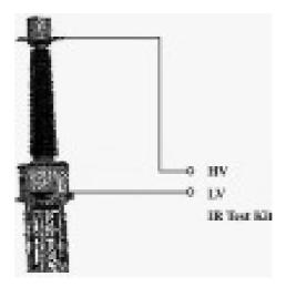
Figure 7 - Typical Arrangement for insulation resistance (IR) measurement
