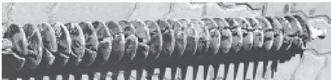
Figure 2 – Composite insulators used on the strung busbars eroded to the core in under two years
