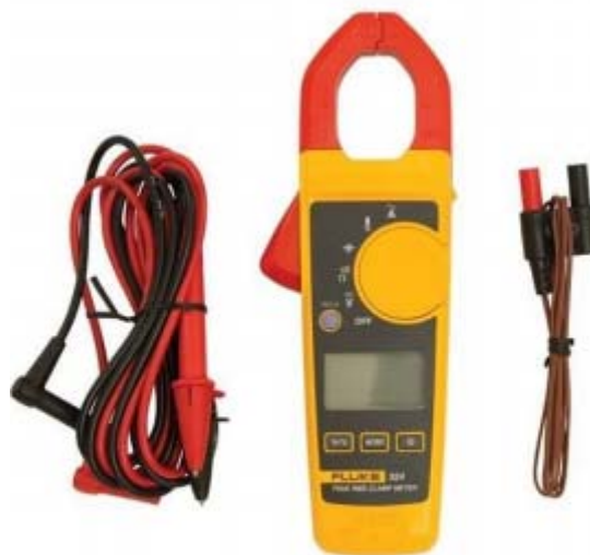
Figure 12: Clamp meter with its components
