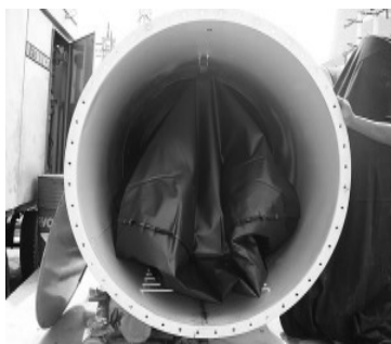
Liquid conservator with rubber diaphragm
