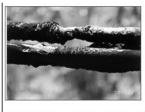
Figure 4: Burnt Outer Sheath
