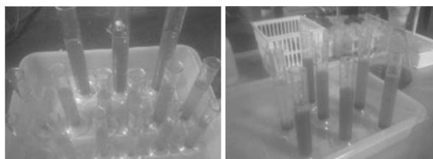
Fig. 2. Settling of microalgae on effect of coagulants
