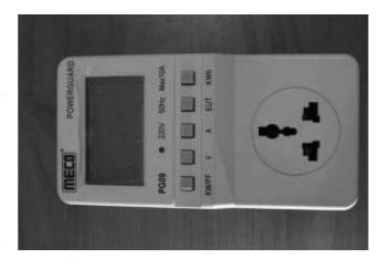
Fig.1.Powerguard meter for PF measurement B.Total Harmonic Distortion(THD)
