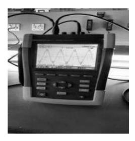
Fig.3.Flukemeter showing Total Harmonic Distortion
