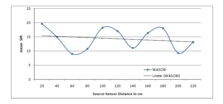
Fig 2: Mean SIR of separated components with WASOBI algorithm for various source-sensor distances
