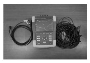
Fig.2.Flukemeter for Power quality indices measurement
