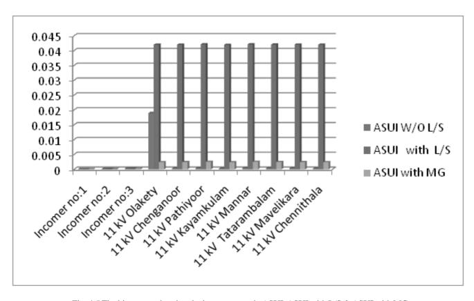
Fig. 4.5 The histogram showing the improvement in ASUI, ASUI with L/S & ASUI with MG
