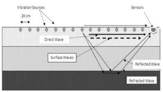
Fig 1: General Arrangement of field data Collection
