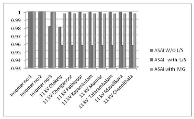
Fig. 4.4 The histogram showing the improvement in ASAI,
