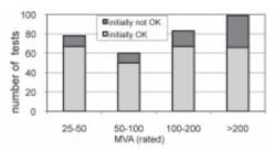
Fig. 7: Initial power transformer failure rate for various ranges of MVA rating
