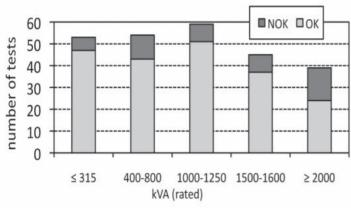
Fig. 11: Test failure statistics of distribution life, more precisely: the 90 transformers
