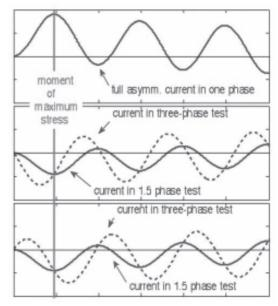
Fig. 4: 1.5 Phase test method showing that at the moment of maximum stress, the current in all phases is identical to a full three-phase condition.
