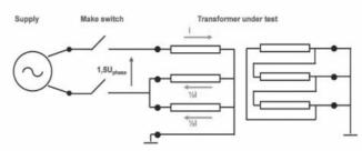
Fig. 5: Test-circuit for 1.5 phase short-circuit tests.
