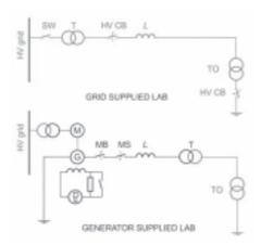
Fig. 3: Lay-out of grid- and generator supplied test laboratories. T: laboratory transformer, TO: transformer under test; HV CB: high-voltage circuit breaker, MB: master breaker, MS: making switch, G: generator, M: motor, L: reactor
