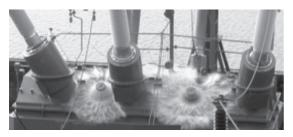
Fig. 10: Oil spill upon short circuit application
