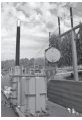
Fig. 6: Short-circuit test of a 800 kV class transformer
